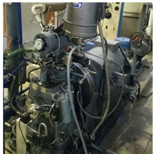
Picture 3: Experimental setup for nano-additives in a diesel engine [6].
