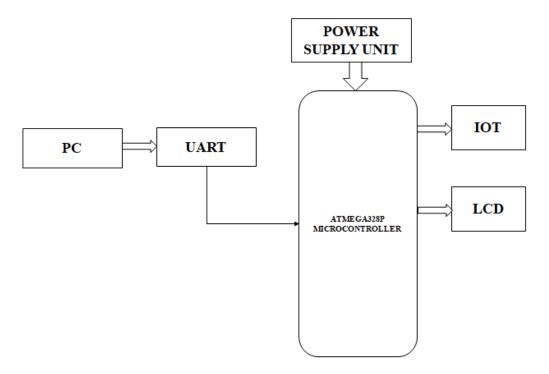
**UART** (**Universal Asynchronous Receiver-Transmitter**): UART is a hardware communication protocol used for serial communication between microcontrollers and peripheral devices. In the system, UART facilitates communication between the Arduino Uno microcontroller and other components such as sensors and modules.
