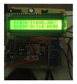
And if the temperature rises above 100 degree the alarm will be generated the below image show experimental value of temperature sensor
