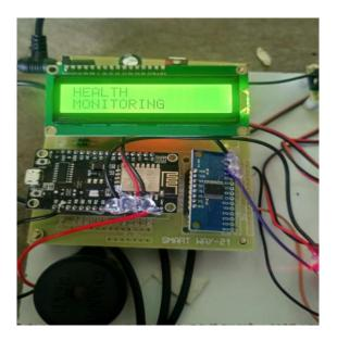
In the LCD Display it will display the temperature, Blood glucose level, Blood Oxygen level and Pulse rate of the patient that is shown below:
