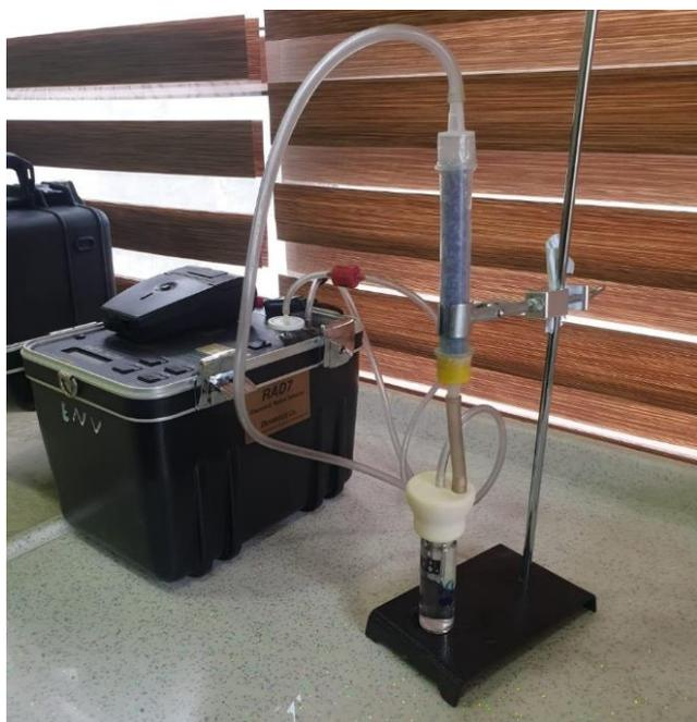
**Fig.3** RAD7 Detector Setup with RAD-H2O Accessories used in this study
