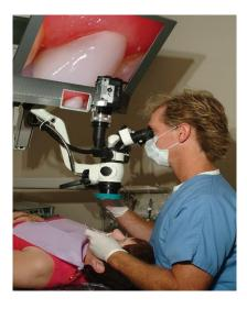
**SUPPORTING STRUCTURE-** Ensuring stability during operation, the supporting structure can be floor, ceiling, or wall-mounted, allowing for precise maneuverability, especially at higher magnification levels.<sup>40</sup>
