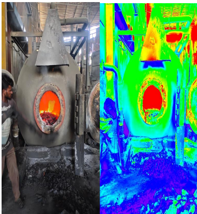
Fig.4.1 and Fig.4.2 ROTARY FURNACE'S THERMAL IMAGES.
