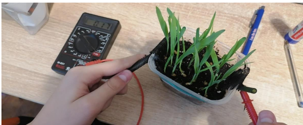
Fig.1. Plant-microbial fuel cell
