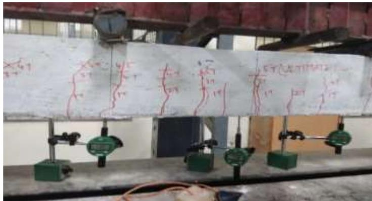
Fig. 6 Beam crack patterns.
