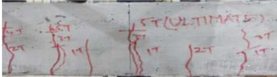
**Fig.11 Concrete TOPS beam crack behavior**
