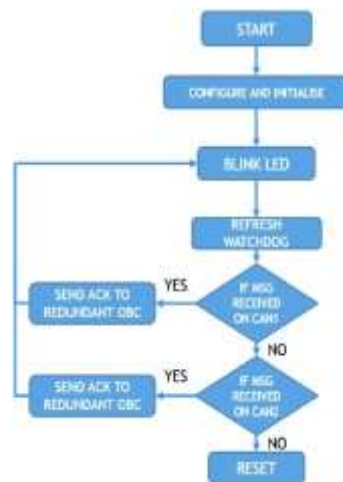
Figure 6: Flow Chart of Master OBC
