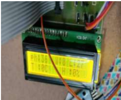
Fig 3: LCD showing pH, Water level, Temperature, Humidity
