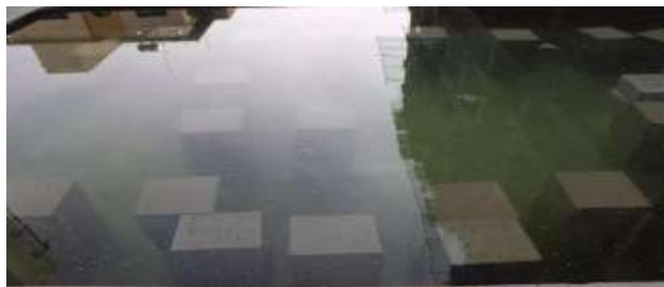
Fig. 3: Curing of cubes
