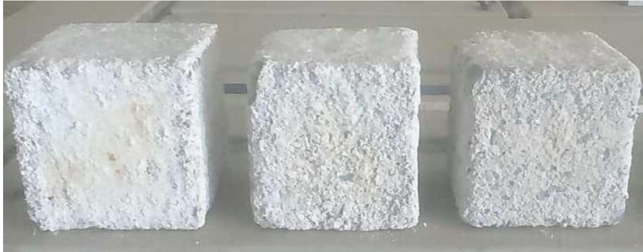
Fig. 4: Acid attack on concrete
