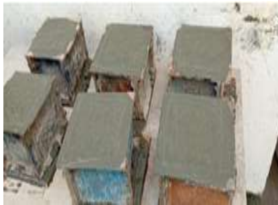
Fig. 2: Casting of cubes
