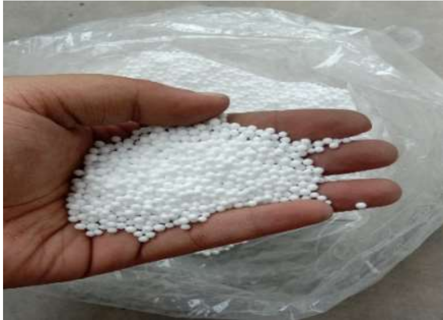
Fig. 3: EPS from the factory
